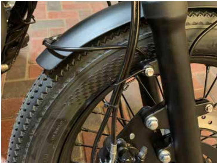
D 1.5 Check routing of cables and wiring, handlebars move freely
