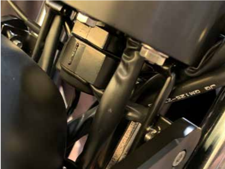
B 1.5 Check routing of cables and wiring, handlebars move freely
