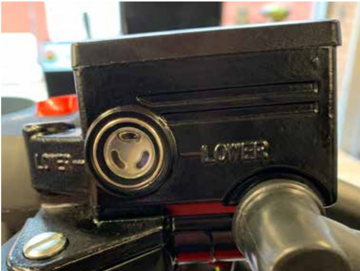
F 1.6 Check brake fluid levels (front & rear), top up if necessary
