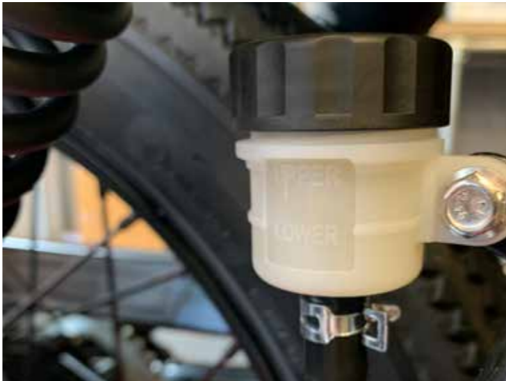
G 1.6 Check brake fluid levels (front & rear), top up if necessary
