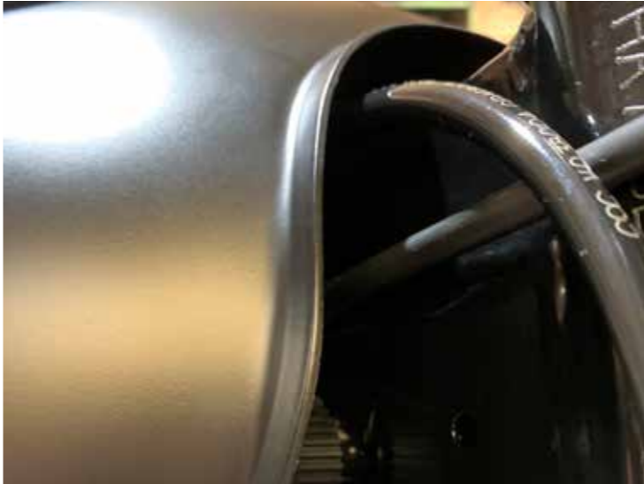
C 1.5 Check routing of cables and wiring, handlebars move freely
