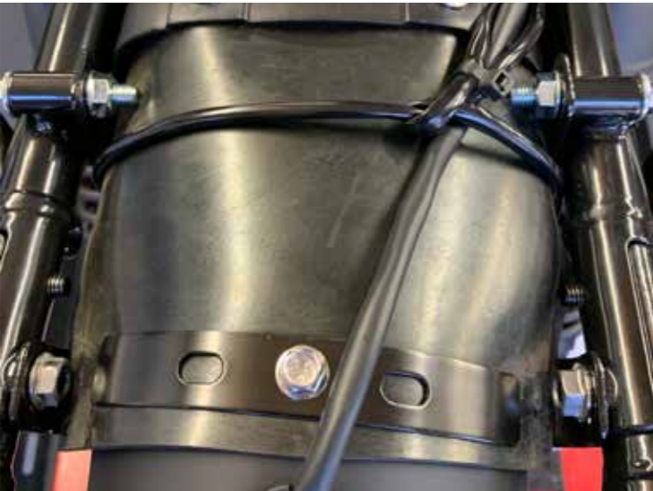
E 1.5 Check routing of cables and wiring, handlebars move freely
