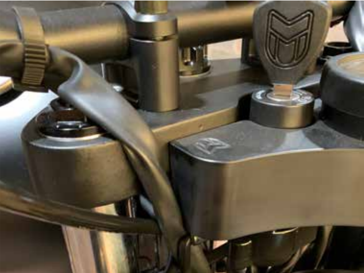
A 1.5 Check routing of cables and wiring, handlebars move freely
