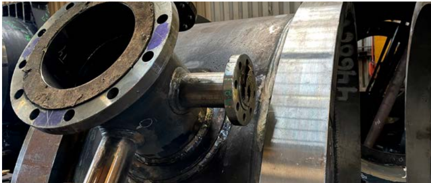
Example of really tight flange – NBFF is the only tool suitable here.
