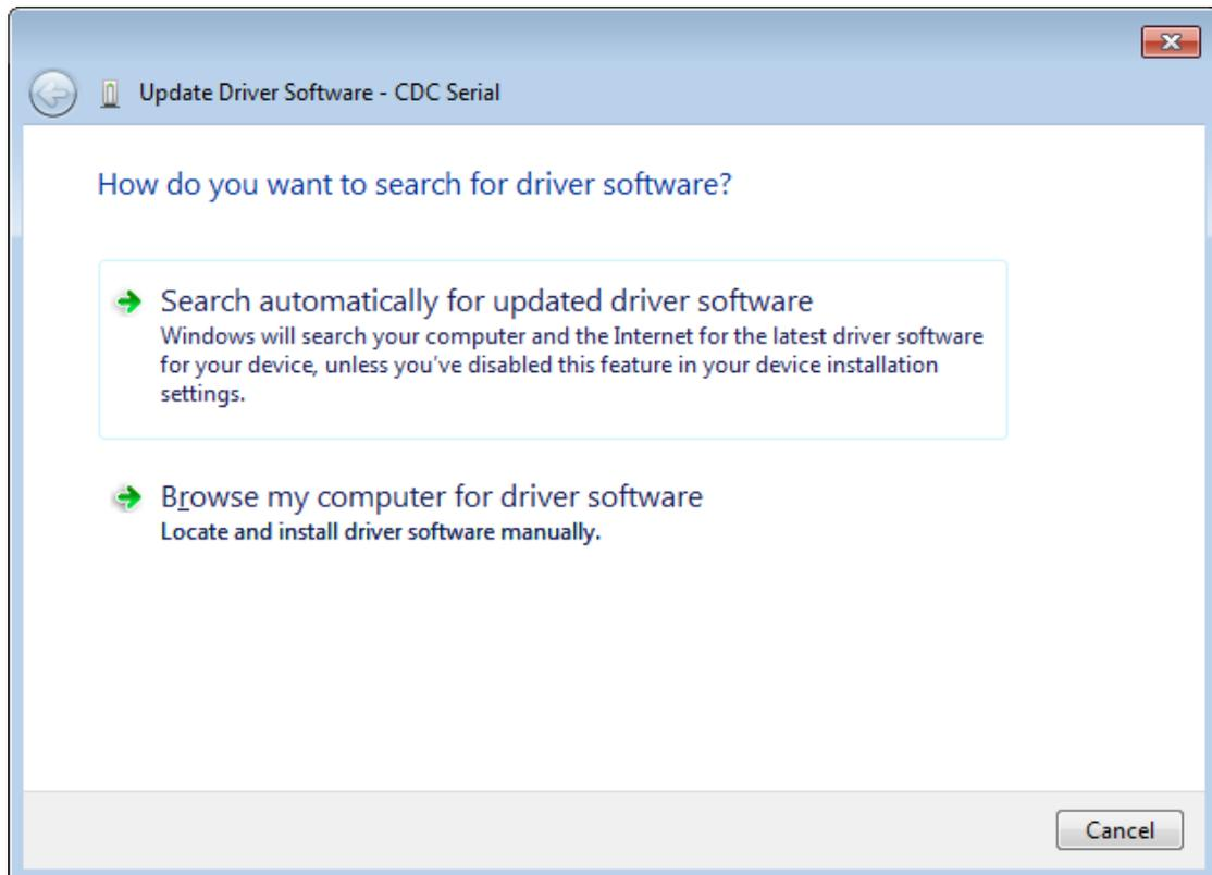
6. Manually search the driver path and select the location where the driver installation package is placed. Click the **Next**.
